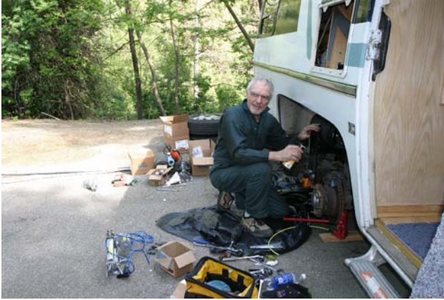
Frank Installing Four Airbag System (FB)
