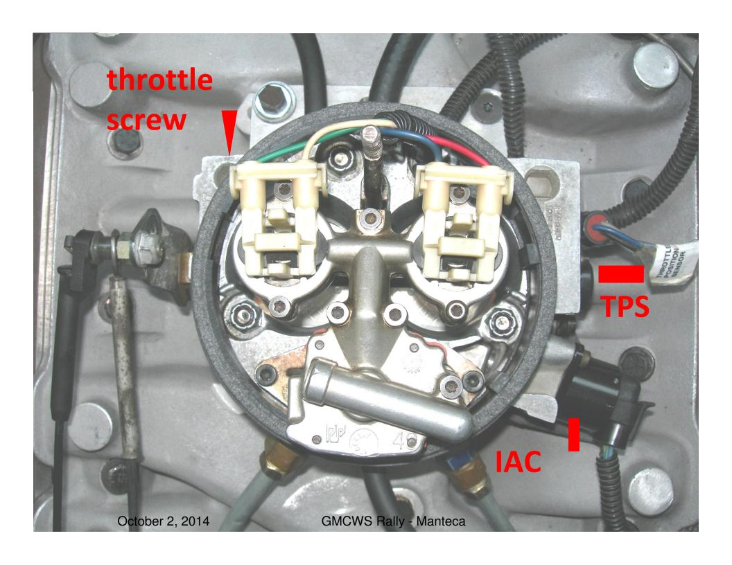
The diagram below shows how the IAC control will by-pass the air around the throttle valves when the chip controls the IAC and the idle speed. In doing the calibration, we are going to move the IAC pintle into the seat, shutting off any by-pass airflow, and then disable the IAC. Then we will adjust the throttle plates for "minimum idle" speed.
