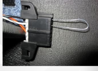
3- Turn key to ON, do not start engine, wait 8 seconds. This will extend the IAC pintle and close off the air passage in the body of the TBI.
