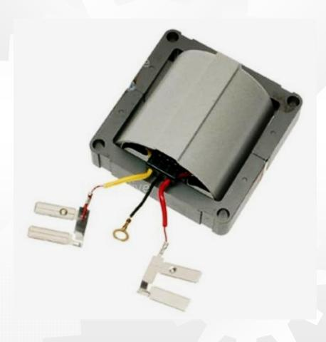
The <u>pick-up pole</u> piece needs to match the ignition coil. The <u>WHITE</u> wire needs to be closest to the locator lug that index's the pole piece to the distributor. The wires will have a <u>YELLOW</u> connector or cable tie.
