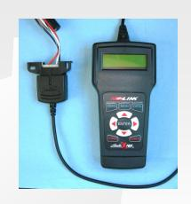
If you have installed the EBL system then you can use the sensor diagnostics page of the WUD to view the sensor info needed to do the calibration.
