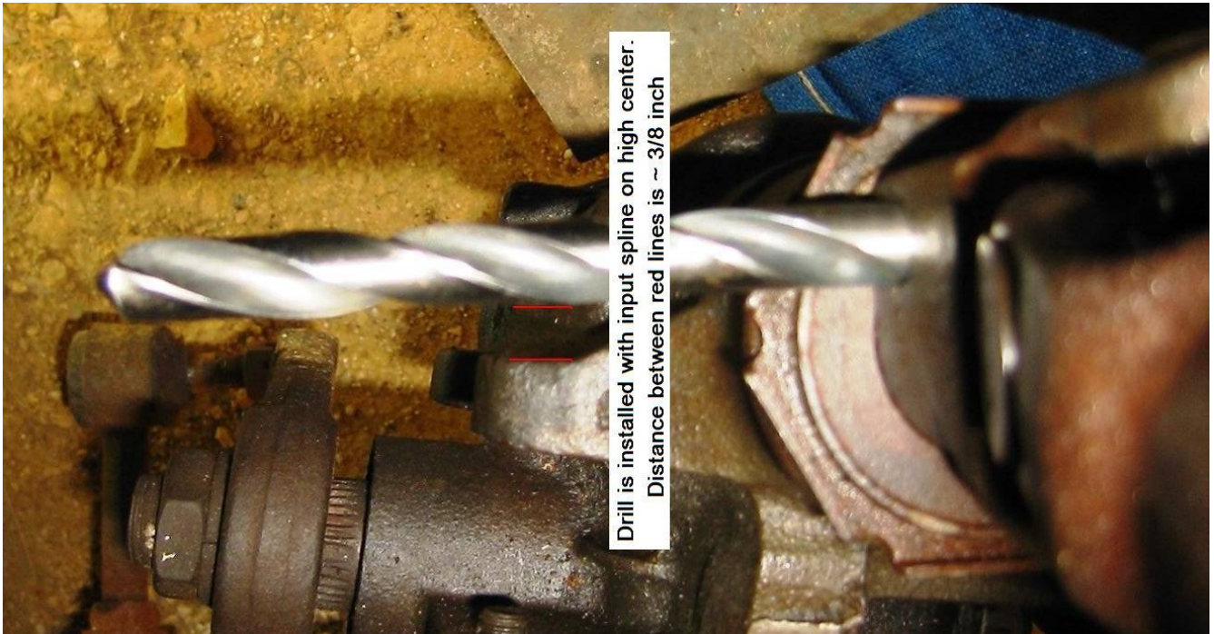
Figure 3 – Yoke bolt position – 29/64ths drill installed
