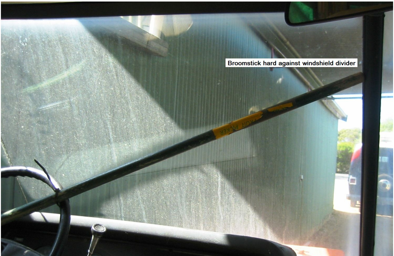
Figure 6C – Broomstick installed to keep steering wheel from turning
