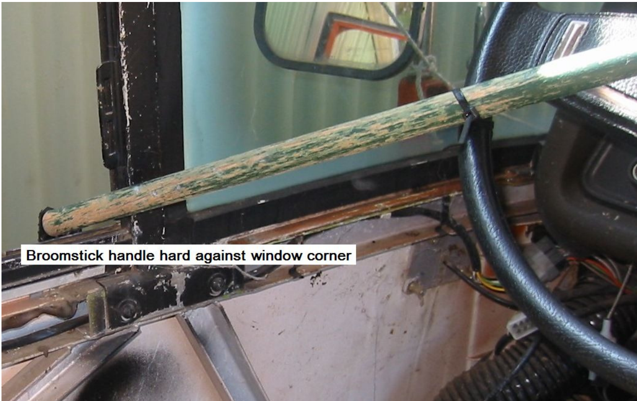
Figure 6B – Broomstick installed to keep steering wheel from turning
