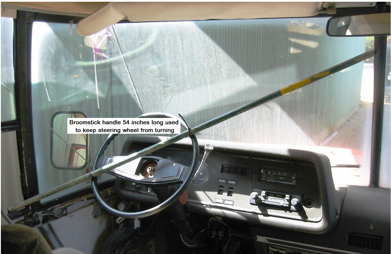
Figure 6A – Broomstick installed to keep steering wheel from turning
