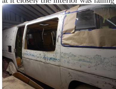
The cockpit floor is rotted under both side windows. All the cabinetry needs to be rebuilt. Side windows needed new felt. No way to put lipstick on this Pig. But did I say, it has a Caddy 500?
