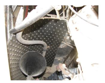
Driver's side outside – grill is on left and top of the photo. Deflector is held in place by the same bolt that hold the hydraulic line to wiper motor. Front is not secured.
