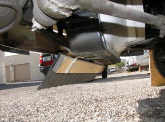
Air dam from left-front. Mud flap material is screwed to support bar.
