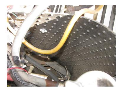
Passenger side outside – grill is at top right in photo. Used a bolt to attach it to the side of the radiator bracket in one place. Front is not secured.
