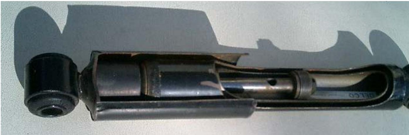
This is the original AC/Delco that came with the Motorhome. It's a twin tube design. Inner tube chamber. It is no longer made
